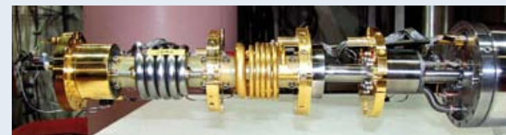
Dilution refrigerator capable of cooling samples to the milli-Kelvin temperatures, required to observe novel quantum effects in nanostructured samples.
