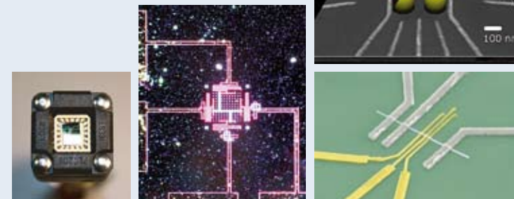
Left: Samples with nanostructures are bonded onto a chip-carrier and measured at low temperatures.
